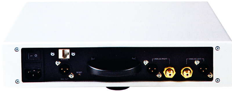
ABOVE: Power switch is at the rear. Both single-ended (RCA) and balanced (XLR) fixed level analogue outputs are provided, and an AES/EBU (XLR) digital output
