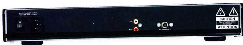
ABOVE: Aerial and power in, left; and audio out, right. Simple and functional but having the rear mounted mains switch is something of a nuisance
