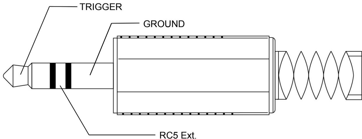
On the back panel of MyAMP you will find a 2.5mm diameter jack input indicated by : TRIG / IR-IN. Following the diagram above you can remotely turn MyAMP in and out of Standby by sending between GROUND and TRIGGER a positive DC voltage with a value between 5V and 12V.
